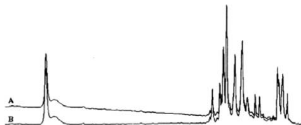
Figure 1. In spectrum B (flat baseline), the Euclidean Distance algorithm should yield good results. In spectrum A (sloping baseline), the First Derivative algorithm should yield good results.
