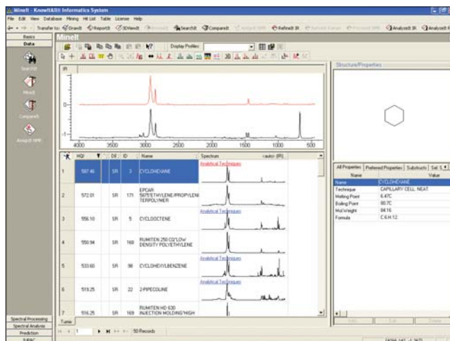
Figure 1. Full spectrum Euclidean search of the test spectrum against the 200 compound SR demo database.
